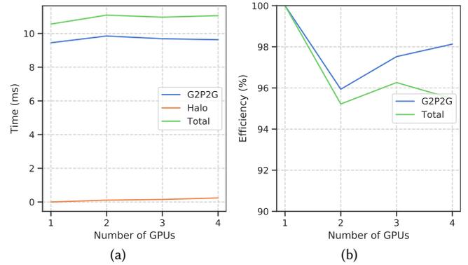
**Fig. 13. Weak scaling; side-by-side layout.** (a) The per time-step wall time remains steady with an increasing number of GPUs for the  $G2P2G$  and overall performances. The additional overhead of halo tagging is growing but remains insignificant. (b) Both the  $G2P2G$  kernel and the overall efficiencies stay above 95% even when employing 4 GPU devices.
