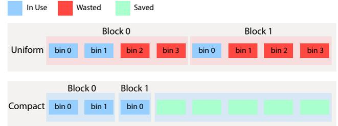
Fig. 8. **Compact storage.** Particles are often unequally distributed in space. Hence, uniformly allocating fixed memory space for each particle block would result in a significant amount of unused memory. Instead, a more efficient strategy is to allocate just enough particle bins for each block according to the current distribution of particles.
