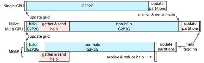
Fig. 9. **Instruction pipelines.** The additional operations in the multi-GPU MPM compared to the single-GPU MPM are displayed in red. By masking these halo-region-related data transfers with the execution of the  $G2P2G$  kernel, one can achieve more optimized scaling results with multi-GPUs.
