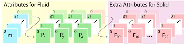
Fig. 7. **Binning.** The internal layout of each particle bin is SoA. In this example, the array length of the particle bin equals to the thread group size on the NVIDIA GPU architecture (*i.e.*, 32 for an NVIDIA GPU warp) for coalesced memory access within a bin. The number of properties is flexible according to the material; we used 4 for fluids and 13 for solids.
